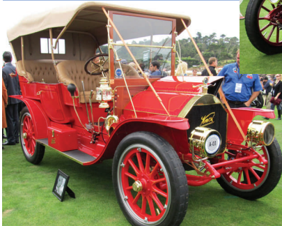
1906 Adams-Farwell 6A Runabout This car is unique with its air-cooled 5-cylinder rotary engine.
